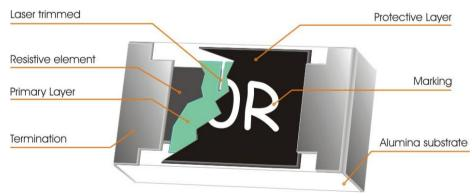
Fig 1. Construction of 2512, 2010 Chip-R
