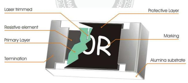
Fig 1. Construction of Chip-R WFxxB
