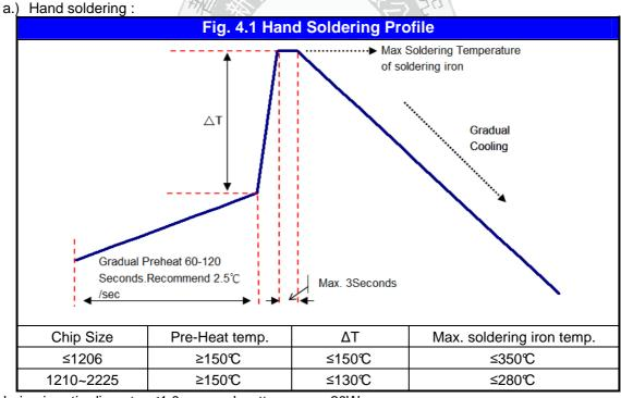
\* Soldering iron tip diameter ≤1.0 mm and wattage max. 20W.
